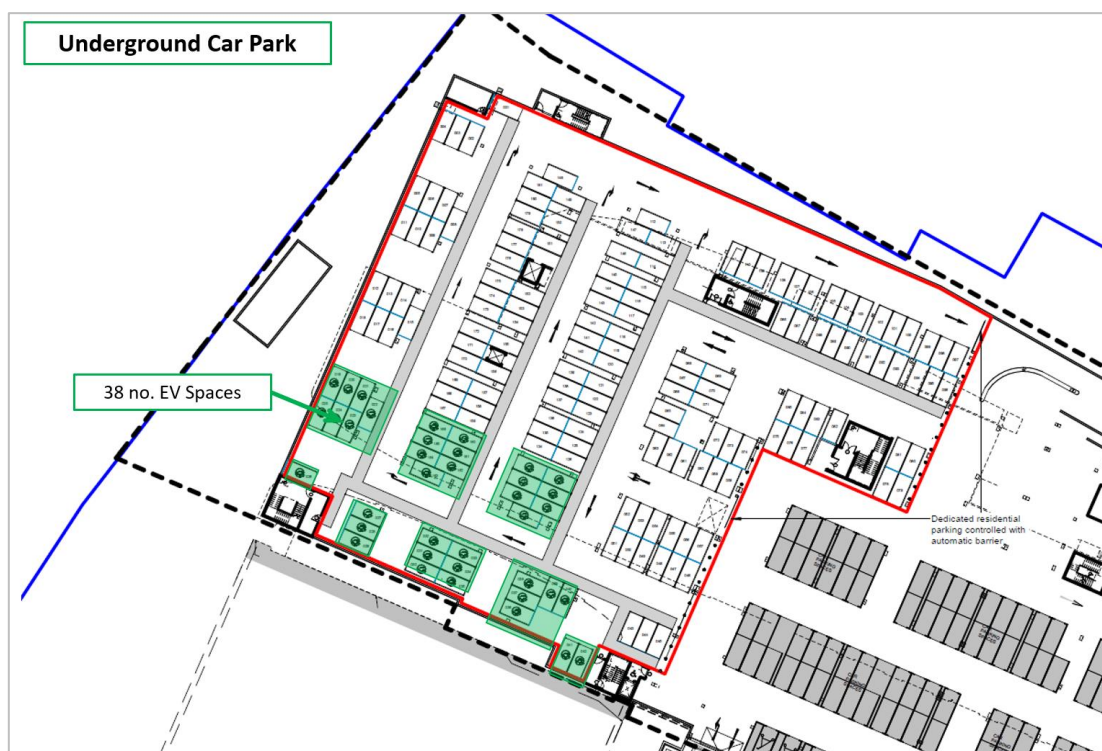
Figure 4-15: EV Car Park Spaces in Underground Car Park
